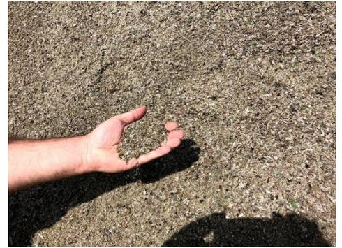
Glass is fed into a “cone” which crushes the glass, and conveys it through two screens. About 25-35% of the material is disposed as “overs”, except the ferrous fraction, which is separate with a magnet. The final output is ¼” minus, which is usually mixed at 1% into course gravel.
